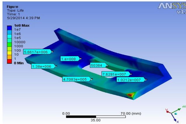
Figure 11: Fatigue Life of the Hole(80mm)
