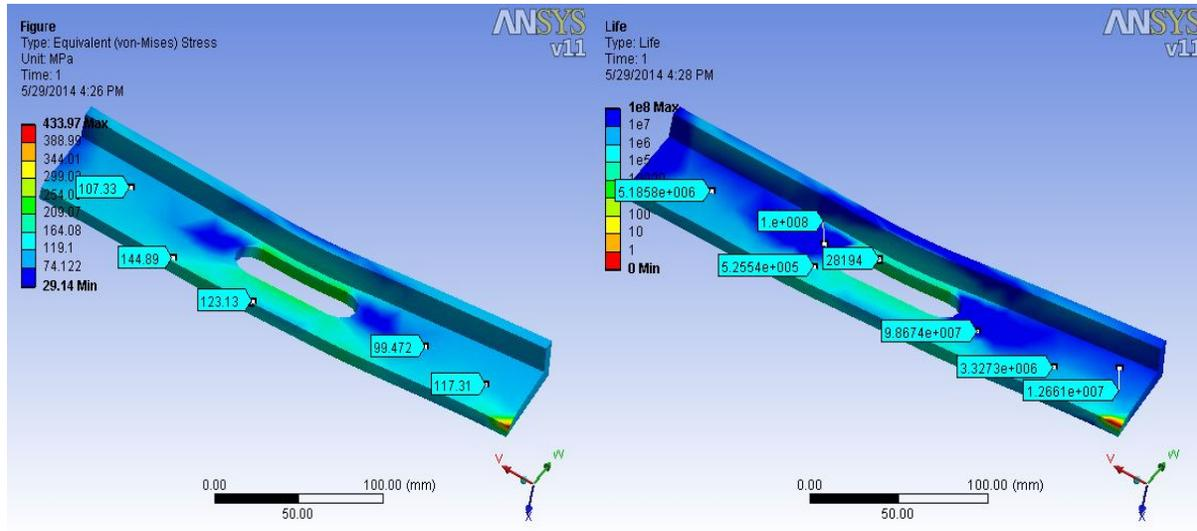
**Figure 7 Equivalent stress or von mises stresses(50mm Hole) Figure 8: Fatigue Life of the hole(50mm Hole)**
