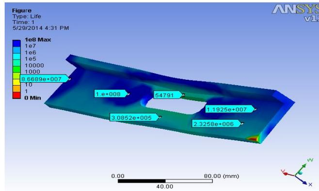
Figure 9: Fatigue Life of the Hole(60mm)
