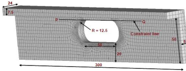
**Figure 6: Geometric dimensions (in mm) and a half finite element model of the stiffener structure (the boundary of the vent hole is not allowed to move beyond line PQ).**
