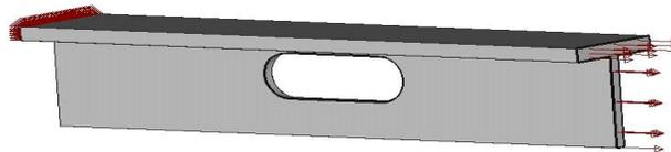
Figure2: Half finite element model of the stiffener structure
