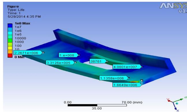
Figure 10: Fatigue Life of the Hole(70mm)
